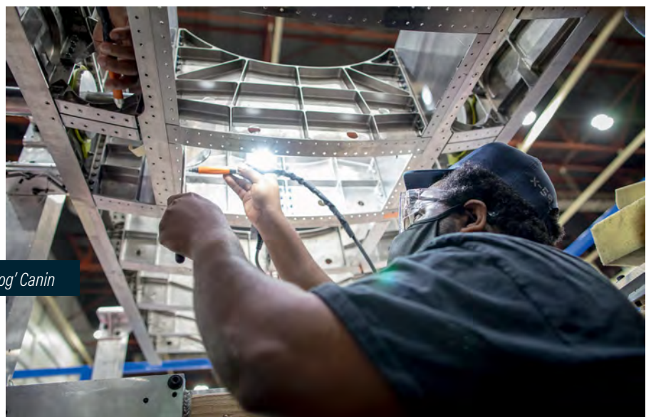
ABOVE: The X-59’s cockpit section is a unique feature of the aircraft. Shown here during production, space has been made for its side windows but not a forward cockpit window – because there isn’t one. Instead, the platform will employ NASA’s innovative XVS suite.
