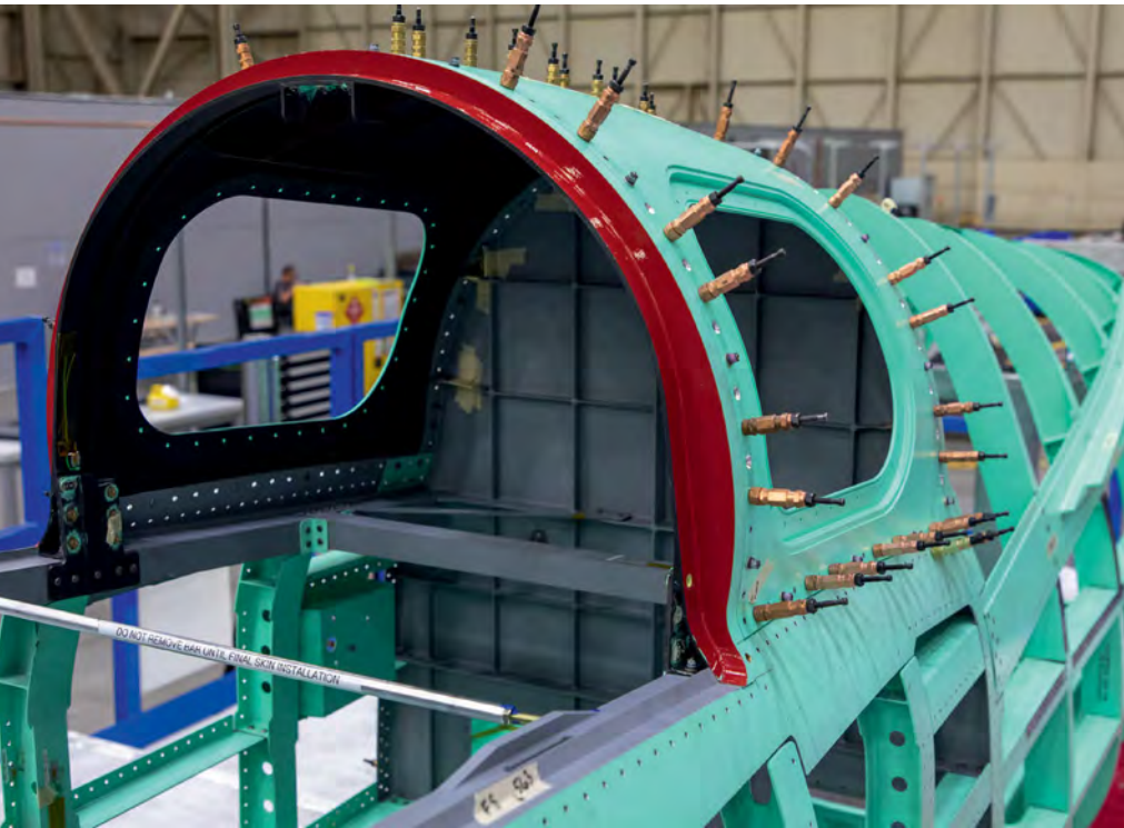
ABOVE: The X-59’s cockpit section is a unique feature of the aircraft. Shown here during production, space has been made for its side windows but not a forward cockpit window – because there isn’t one. Instead, the platform will employ NASA’s innovative XVS suite.
