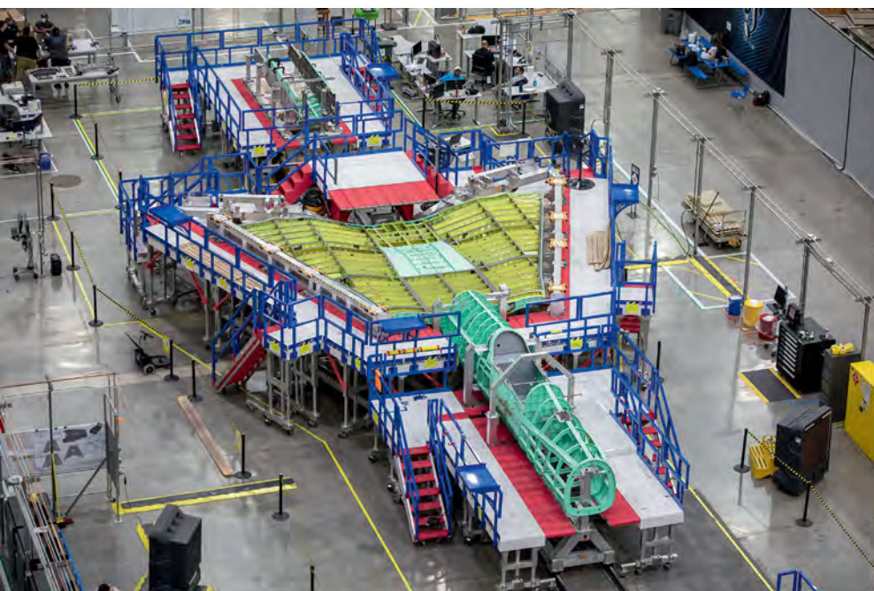
LEFT: In June 2020, engineers and technicians at Skunk Work attached the QueSST's wing and cockpit sections together.
