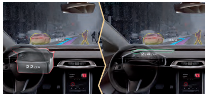
FAR RIGHT Compact waveguide AR HUD
